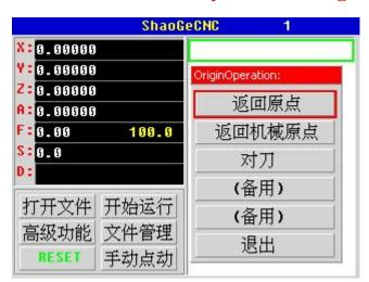
"Return to origin" Z-axis height to rise to safety, XY axis back to the origin, Z-axis and then passed back to the origin.
